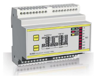
**RI-R60** is a device that allows to control the insulation to earth in alternating neutral networks up to 760 V (IT systems) in direct insertion and in network up to 1000V with ARI-R60 adapter.
